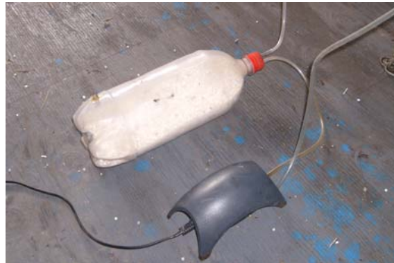
Desiccant and pump with return airline.
