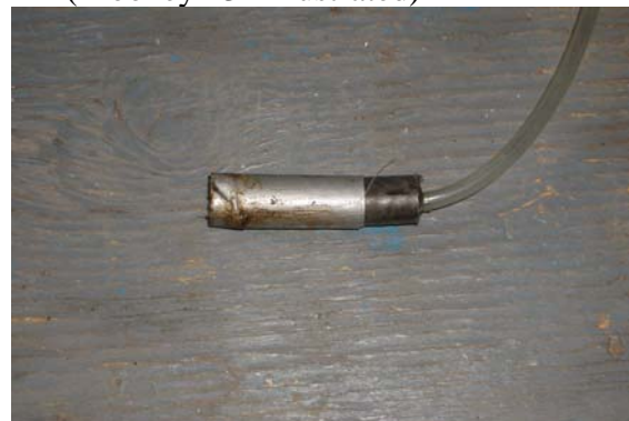
Blow-by return rubber fitting
