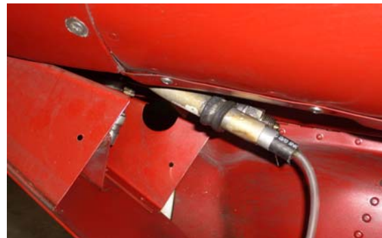
Pump return line installed in Blow-by port (Mooney 231 illustrated)
