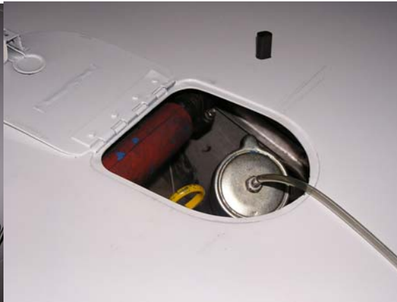
Air inlet fitting in oil filler cap
